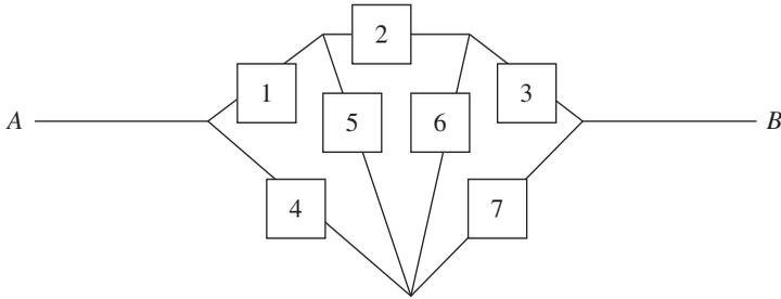
The system as a whole is working if water flow from point  $A$  to point  $B$  is feasible through working pumps.
