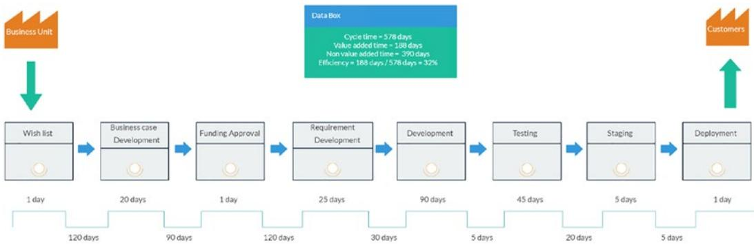
**Figure 15-6.** Value stream map for a software development process
